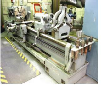
NEBEL, MODEL HD, 30" X 96" CC, 21" 4 JAW CHUCK, 2" HOLE THRU, 20-2516 RPM, TAILSTOCK, (2) STEADY RESTS, FOLLOW REST, THREADING, KDK TOOL POST, S/N 8906
