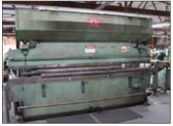
CHICAGO 1214-C PRESS BRAKE, 12' X 75 TON, FRONT OPERATED MANUAL BACK GAGE, S/N L-17445
