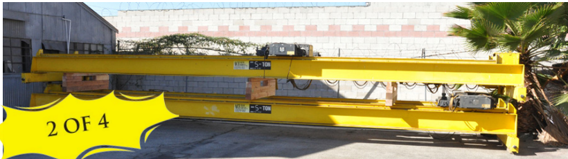
5 Ton x 39' Used Spacemaster Over Riding Double Girder Bridge Crane, Mdl. JobS-13162, Pendant
