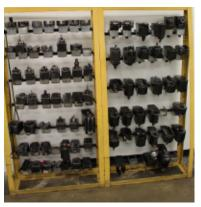
LARGE MODULAR STORAGE CABINETS FULL OF: INDEX & BROWN & SHARPE CAMS, COLLETS, FIXTURES, BUSHINGS, CUT-OFFS, HOLDERS AND REALTED TOOLING/PARTS
