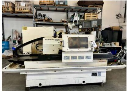
MITSUBISHI RC32-B50A, PLAIN OR ANGLE HEAD, FANUC SERIES 16-GC CNC CONTROL, 12.6" SWING, 19.7" CENTERS, 18" DIAMETER WHEEL, 7.3 HP WHEEL POWER, 1800 RPM, S/N GJ543
